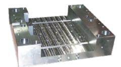
RoyAlloy plate shown after extensive pocket milling measured only 0.006" (0.15mm) distortion from corner to corner – plate size 6" x 28" x 32" (152mm x 711mm x 813mm).
