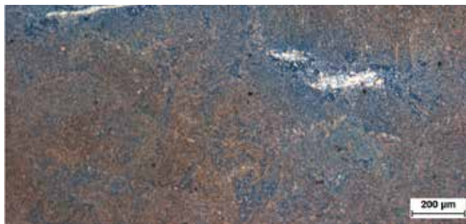
DIN-Number 1.2316 Martensitic structure with delta ferrite content
