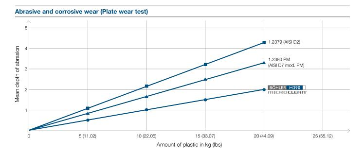
Plastic: Polyethersulfon (PES), Trade name: Ultrason E2010G6, Glass fibre content: 30 wt.%, Temperature: 400 °C (750 °F)
