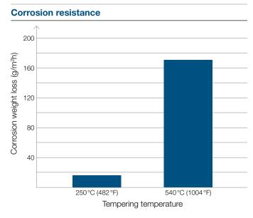
For highest corrosion resistance use lower tempering temperatures. Heat treatment: austenitizing at 1150  $^\circ C$  (2.100  $^\circ F)/20 min./5 bar, without subzero-cooling$
