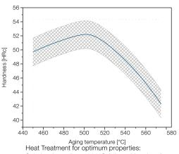
Heat Treatment for optimum properties: Solution Annealing: 1000°C / 1h soaking time / air cooling to room temperature Ageing: 500°C / 3h soaking time / air cooling
