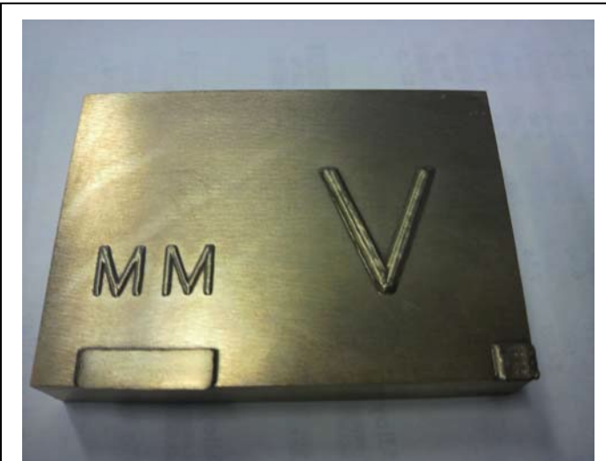
Figure 1. MoldMAX V block laser welded with WeldPAK V filler metal
